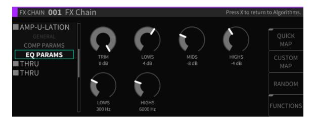
On the H9000, each Algorithm contains a set of parameters; you adjust these parameters to adjust the sound of the Algorithm you have selected.
