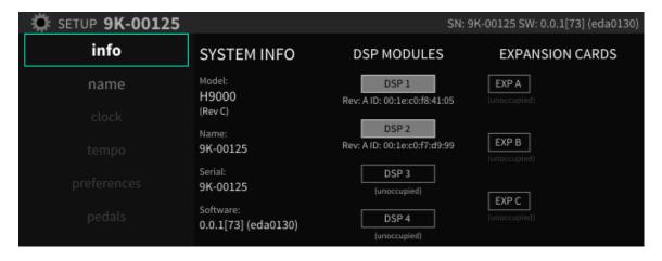
Press the *Setup* button to enter the Setup menus for the H9000. The left-hand side of the display shows a list of different areas you can customize, including:
