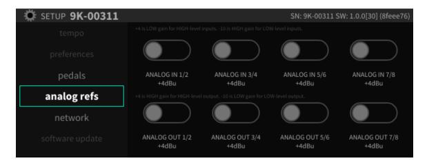
The Analog Reference Levels screen allows you to set the levels for the 8 analog inputs and outputs present on the 25-pin DSUB connector. This allows the H9000 to be installed in a wide variety of environments, and interface at an optimum level with a vast assortment of other equipment.
