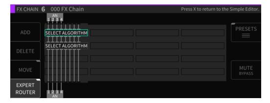
Press the latching *Expert Router* soft key to enter the "Expert Routing" mode. The display switches to a graphical routing matrix, where you can view and edit a high level overview of:
