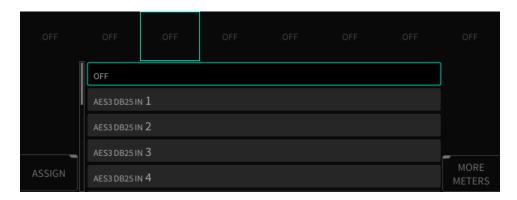
On a stock H9000 unit with no expansion cards installed, the following single input/output channels can be assigned to the meters:
