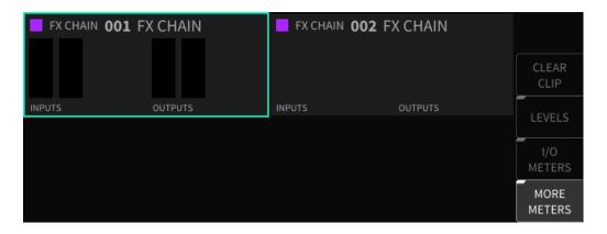
Press the latching *More Meters* soft key to enter the *More Meters* screen; the display changes to show metering data for the currently loaded available FX Chains.
