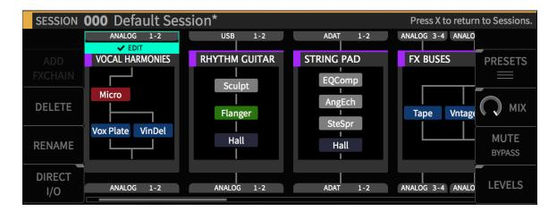
Press the front panel *FX Chain* button to switch the display to the *FX Chains* screen, where you can view and edit the various FX Chains of the currently loaded session.
