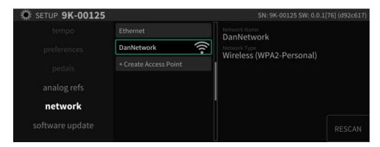
Navigate to the wireless network you wish to connect to and press the *Enter* key.
