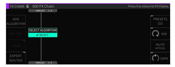
In the H9000, each FX Chain can contain up to four separate signal-processing Algorithms. The *Algorithms* screen is where you work with these specific algorithms; you can navigate to it by either:
