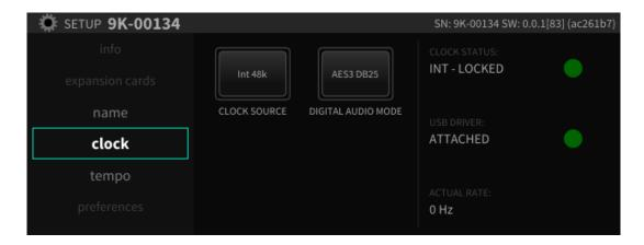
The clock setup menus allow you to set the unit's sample rate and MIDI Clock tempo. Available settings include:
