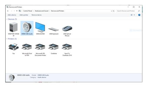
The H9000 will now appear as an audio device in the Windows "Devices and Printers" control panel, and its audio inputs and outputs can be used from any ASIO compatible software.
