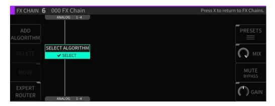
• Use the navigation controls to select an Algorithm. Each entry contains helpful info (Ins/Outs, a description of the algorithm, tips on its use, etc.).
